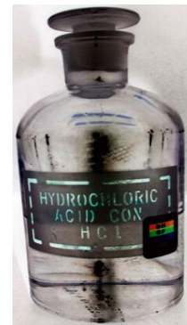
HCL 5% for clean sensor
