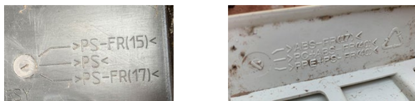
Figure 2-2: Resins and FR Markings on e-waste plastic parts
